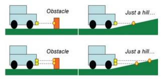
**Figure 7.** Obstacle or hill? With a single planar LIDAR, obstacles cannot be reliably discriminated from traversable (but hilly) terrain. Multiple planar LIDARs allow appreciable changes in z to be measured, resolving the ambiguity.
