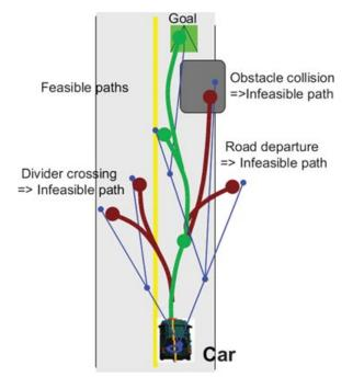
**Figure 22.** Illustration of RRT motion planning. Each leaf of the tree represents a stopping location. The motion control points (line-connected points) are translated into a predicted path. The predicted paths are checked for drivability (curved paths).
