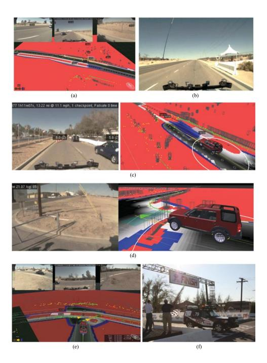
**Figure 34.** UCE highlights. (a) Talos overtaken by traffic vehicle. (b) Talos reaches its target speed of 25 mph (24 shown on the sign) traveling up Phantom East. (c) Talos slows to merge safely behind the Cornell chase vehicle. (d) Talos waits patiently behind a gate that was blown across an intersection safety zone. (e) A fast traffic vehicle is detected early by radars, and correct intersection precedence keeps Talos in the race. (f) Mission accomplished.
