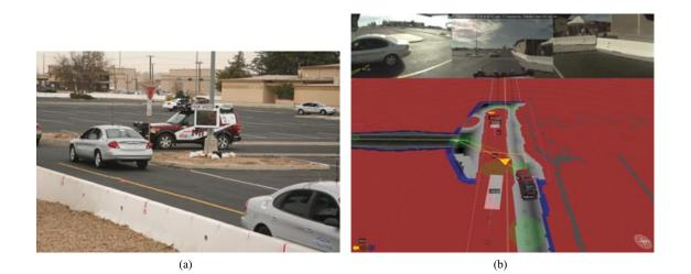
**Figure 31.** Area A second trial highlights. (a) Talos is looking for smaller gaps than in the first trial. (b) The RRT planner is working while waiting for oncoming traffic to clear.
