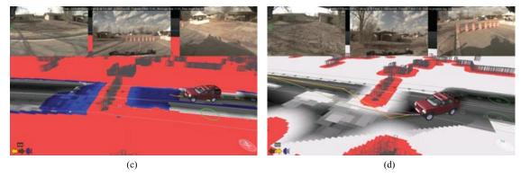
**Figure 27.** Area C first trial highlights. (a) Intersection precedence with four traffic vehicles. (b) Queuing before an intersection. (c) Attempting to go around a blockage. (d) Fail-safe mode 1 permits the vehicle to go around the blockage.
