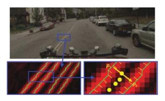
**Figure 16.** Progression from original image through smoothed gradients, border contours, and symmetric contour pairs to form centerline candidate.
