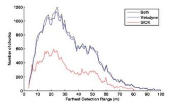
**Figure 11.** Detection range by sensor. For each of 40,000 chunks, the earliest detection of the chunk was collected for each modality (Velodyne and SICK). The Velodyne's performance was substantially better than that of the SICK's, which observed fewer objects.
