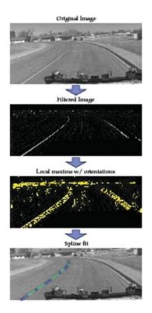
**Figure 15.** The matched filter–based detector from start to finish. The original image is convolved with a matched filter at each row (horizontal filter shown here). Local maxima in the filter response are enumerated and their dominant orientations computed. The figure depicts orientation by drawing the perpendiculars to each maximum. Finally, nearby maxima are connected into cubic hermite splines.
