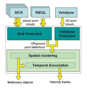
**Figure 5.** LIDAR subsystem block diagram. LIDAR returns are first classified as "obstacle," "ground," or "outlier." Obstacle returns are clustered and tracked.
