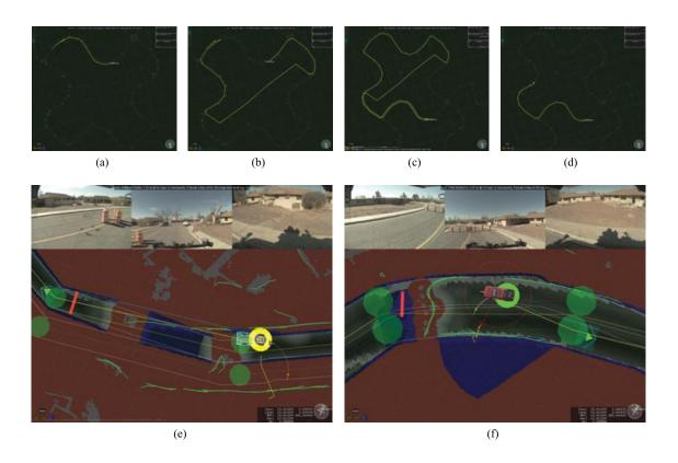
**Figure 29.** Area B second trial highlights. (a), (b), (c), and (d) show a sequence of navigator plans. After a blockage is declared in the gauntlet, Talos attempts to reach the checkpoint from the opposite direction. (e) Talos gets stuck and cannot go into passing mode due to a poor lane estimate resulting in the appearance that it was not entirely in its lane. (f) This blockage was real. Talos detects the blockage and completes a K-turn.
