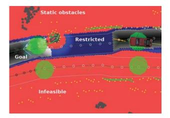
**Figure 19.** Drivability map visualization Arrow (left): Short-term goal location. Light regions (adjacent to the road): Infeasible regions are off limits to the vehicle. Dark region (in front of the vehicle): Restricted regions may be entered only if the vehicle can stop in an unrestricted region farther ahead. Shades of gray: High-cost regions indicate regions accessible to the vehicle.
