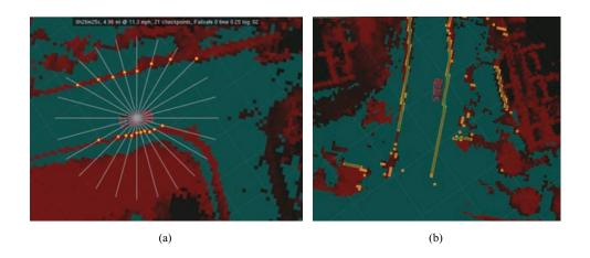
**Figure 13.** Hazard map: Light regions on the road indicate smooth terrain. Dark regions along the road edge indicate uneven terrain such as curb cuts or berms. (a) Rays radiating from vehicle used to detect the road edge. (b) Polylines fitted to road edge.
