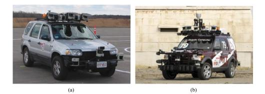
**Figure 3.** Developed vehicles. (a) Ford Escape rapid prototype. (b) Talos, our Land Rover LR3 race vehicle featuring five cameras, 15 radars 12 SICK LIDARs, and a Velodyne LIDAR.
