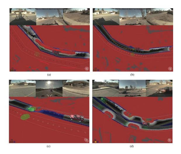
**Figure 32.** Area B third trial highlights. (a) Without visual lane tracking, a curb-free space algorithm localizes the lane. (b) Visual lane tracking often recovers, providing an improved road estimate. (c) Without a virtual obstacle, passing will still occur as long as the object occupies enough of the lane. Here the parked car still induces a passing behavior. (d) Once in passing mode, parked cars are easily maneuvered around.
