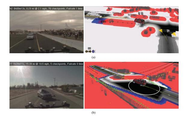
**Figure 20.** (a) An infeasible region is projected down the lane excluding maneuvers into oncoming vehicles. (b) Within an intersection an infeasible region is created between a moving obstacle and the exit matching the velocity direction.
