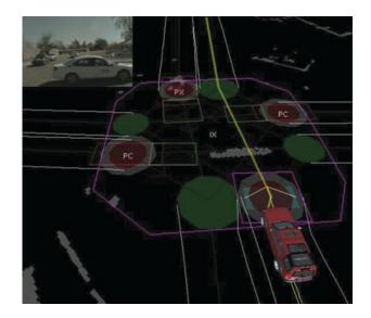
**Figure 18.** The Navigator's view of intersection precedence. PX means that there is a car with precedence at that entrance, and PC means that there is no car or that the car at the stop line does not have precedence. IX means that there is a moving object in the intersection. Talos is clear to proceed when all PX states have transitioned to PC and IX has transitioned to IC.
