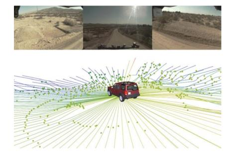
**Figure 9.** Ground model example. On hilly terrain, the terrain deviates significantly from a plane but is tracked fairly well by the ground model.
