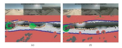
Figure 38. Steep gravel road. (a) and (b) Talos had no problem with gravel roads of gentle slope. (c) Roll-off of the gravel road appears hazardous in the curb hazard map. (d) A phantom curb is detected at the road crest. (e) and (f) Phantom curb detections contort the road corridor, choking the drivable region.
