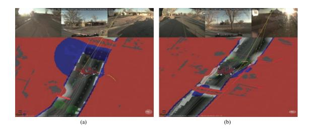
**Figure 33.** Area C third trial highlights. After correctly detecting the blockage, Talos begins a K-turn. The navigator's plan changes. Talos enters fail-safe mode, drives off-road, and is recovered by the pit crew. (b) After the intervention, Talos resumes, and its second K-turn goes well.
