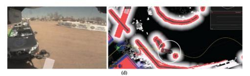
**Figure 40.** Second Caroline–Talos incident. (a) Talos drives around the Caroline chase vehicle. (b) Talos drives around Caroline, which is moving sufficiently slowly to appear as a static object. (c) Talos continues to replan around Caroline, which was perceived as an static object in a different location. (d) Talos continues to drive around Caroline and then initiates an emergency stop, but cannot stop in the space left and collides with Caroline.
