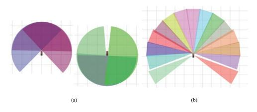
**Figure 4.** Sensor FOVs (20-m grid size). (a) Our vehicle used seven horizontally mounted 180-deg planar LIDARs with overlapping FOVs. The three LIDARs at the front and the four LIDARs at the back are drawn separately so that the overlap can be more easily seen. The ground plane and false positives are rejected using consensus between LIDARs. (b) Fifteen 18-deg radars yield a wide FOV.
