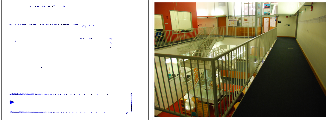
Figure A-8: Partially transparent surfaces. Inferring the correct geometry of a scene is complicated by partially transparent surfaces. Left: the laser data can partially see through the guard rail, detecting both the guard rail and wall on the opposite side. Right: a camera’s view of the same environment.
