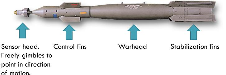
Sensor head detects laser spot in one of four quadrants.
