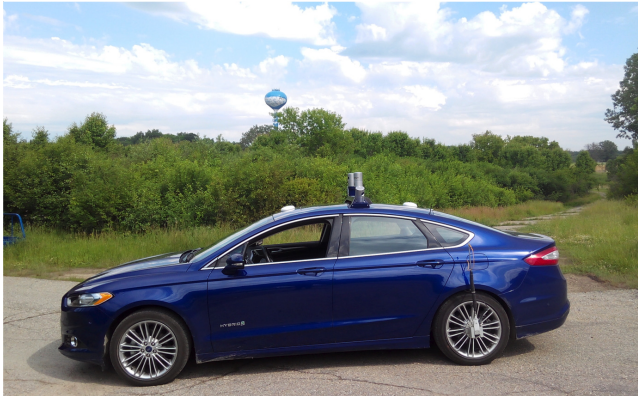
Fig. 4 Our autonomous car platform. The vehicle is a Ford Fusion equipped with a sensor suite including four LIDAR units and survey-grade INS. All perception, planning, and control is performed onboard.
