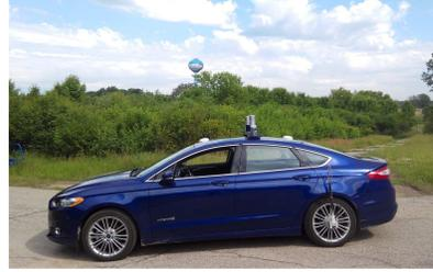
Estimates over the states of other traffic participants are provided by a dynamic object tracker running on the vehicle, which uses LIDAR range measurements. The geometry and location of static obstacles are also inferred onboard using LIDAR measurements.
