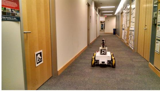
Figure 4.7: The robot platform used for real-world evaluation next to a doorway labeled with an AprilTag.
