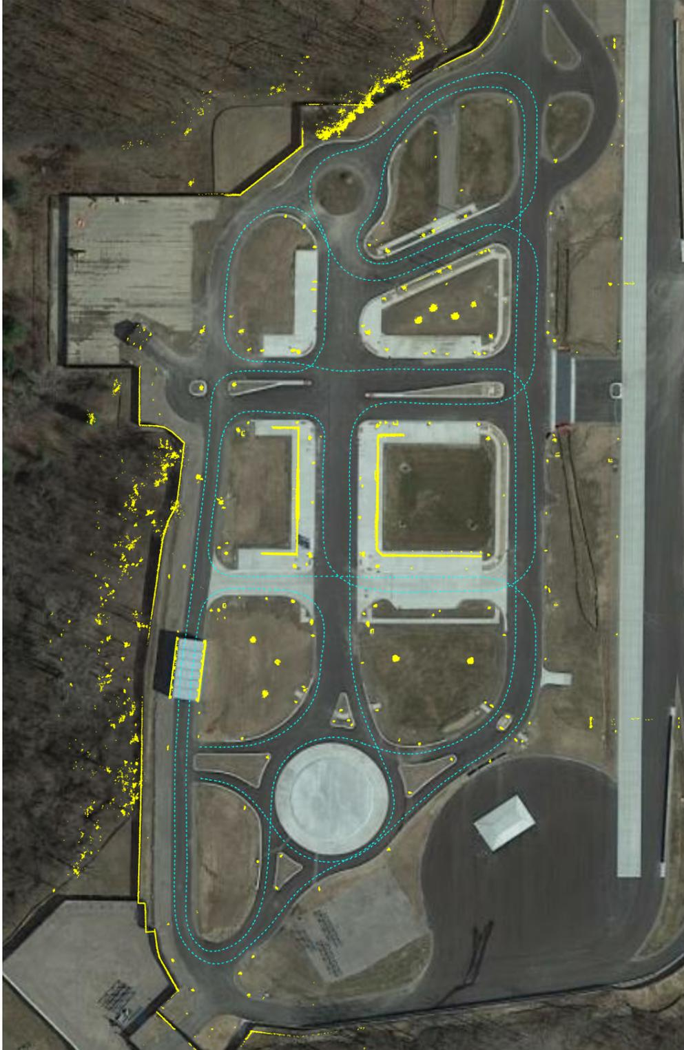
Figure 2.1: A satellite map of MCity overlaid with a 2D metric map of the structure in the environment. The map was built from data collected by driving the route pictured in the environment (cyan) and using LIDAR to detect vertical structure in the environment. An offline SLAM system was then used to construct the maximum likelihood map based on these observations.
