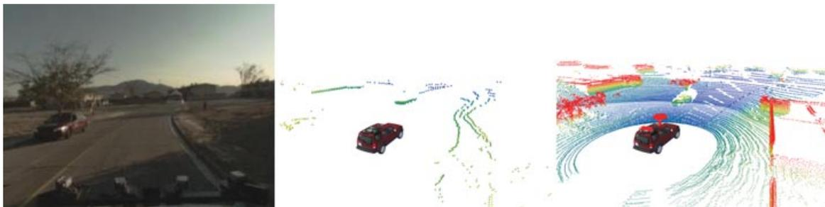
**Figure 6.** Raw data. Left: camera view of an urban scene with oncoming traffic. Middle: corresponding horizontal planar LIDAR data (“pushbroom” LIDARs not shown for clarity). Right: Velodyne data.
