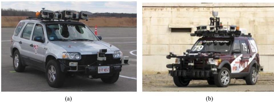
**Figure 3.** Developed vehicles. (a) Ford Escape rapid prototype. (b) Talos, our Land Rover LR3 race vehicle featuring five cameras, 15 radars, 12 SICK LIDARs, and a Velodyne LIDAR.
