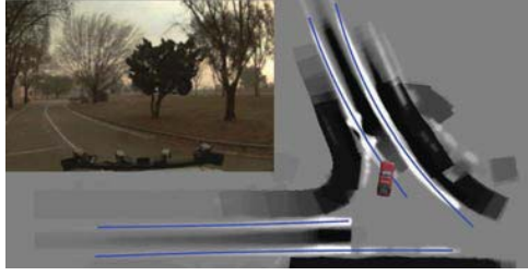
Fig. 17. Our system constructs a centerline evidence image using road edge and road paint detections. Lane centerline candidates (blue) are identified by fitting parabolic segments to the ridges of the image. Front-center camera is shown in top left for context.
