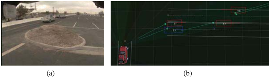
Fig. 12. Radar tracking 3 vehicles. (a) Front right camera showing 3 traffic vehicles, one on coming. (b) Points : Raw radar detections with tails representing the doppler velocity. Red rectangles : Resultant vehicle tracks with speed in meters/second (rectangle size is simply for visualization).
