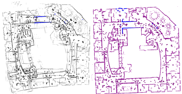
Figure 5. Intel research center. A standard robotics data set before and after automatic loop closures.
