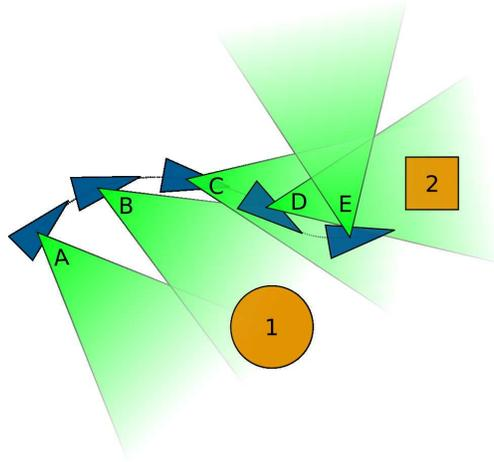
Figure 13: Five images (green) are acquired from a moving robot (blue). For object 1, the camera sharing module returns image *B*, as the object projects fully into image *B* and only partially into image *A*. In contrast, object 2 projects fully into both images *C* and *D*, so the newer image, *D*, is returned.
