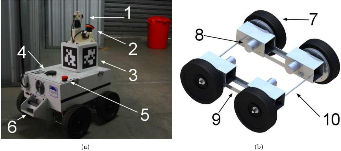
Figure 5: Robot neutralizing a static OOI with relevant components labeled (a): 1. Point Grey color camera, 2. Hokuyo LIDAR unit, 3. APRIL tag, 4. Garmin GPS, 5. Emergency stop button, and 6. 3-in-1 bumper, tip preventer, and handle. The simple suspension was key to our mechanical reliability and included (b): 7. Lawn mower wheels, 8. Motors, 9. Aluminum L brackets (hard attachment) and 10. Torsion bars (soft attachment).
