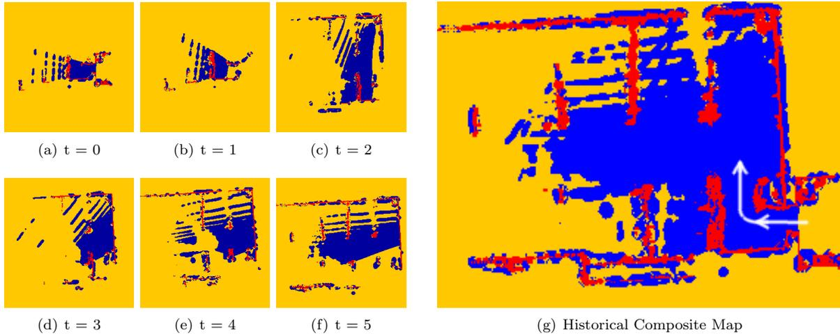
Figure 15: Each of the terrain classification maps (a)-(f) were generated by a single 3D sweep. These sequential maps are merged into a larger composite map (g), which is sent to the path planner. (red indicates an obstacle, blue for drivable terrain, and yellow for unknown)
