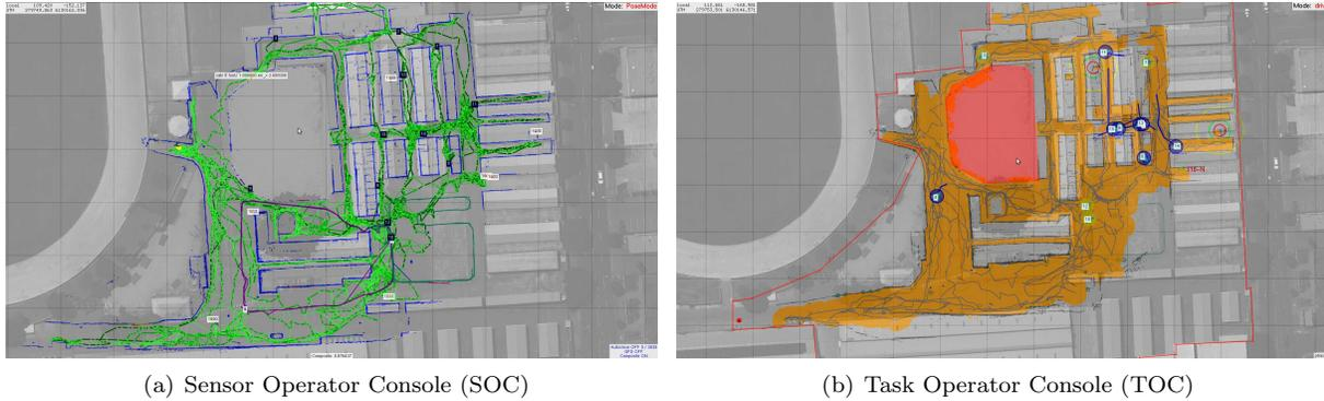
Figure 19: The two interactive displays used by our human operators. The SOC allowed a human to modify override labeled OOIs and to oversee the progress of the SLAM Graph (a). The TOC allowed a human to manage the autonomy of the robots (b). (Best viewed in color)
