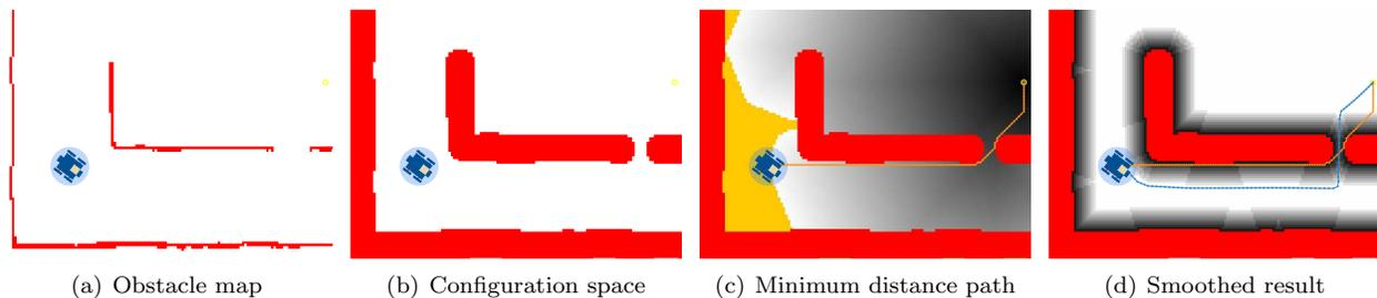
Figure 16: Each stage of on-robot path planning. The configuration space (b) is computed by 2D max disc convolution with the obstacle map (a). The path resulting from Dijkstra’s algorithm (orange) with the distance to the goal for each node examined (gray) are shown in (c). Nodes with distances greater than the solution (yellow) are not examined. Finally, the distance transform (gray) and smoothed path (blue) are shown in (d)
