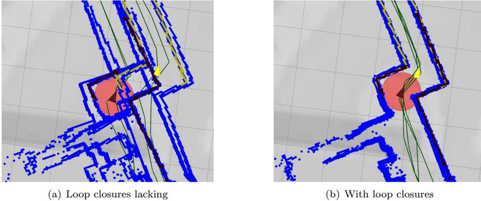
Figure 18: Our maps can typically maintain alignment by running the automatic loop closer, leading to improvement from (a), no loop closures, to (b), with loop closures. When the loop closer fails (not shown), misalignment, such as in (a), can provide a cue to a human operator that intervention may be necessary.
