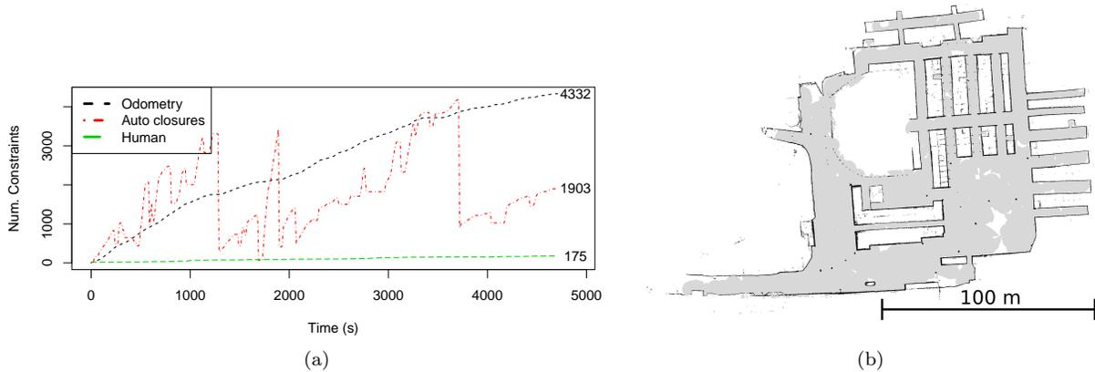
Figure 23: Source of edges in the SLAM Graph during an additional experiment in (a) and the resulting map in (b). Dips in the number of automatically added edges show when the operator used *simplify*, while the increasing number of human-initiated edges shows the interaction rate of the operator to mitigate odometry errors and false loop closures.
