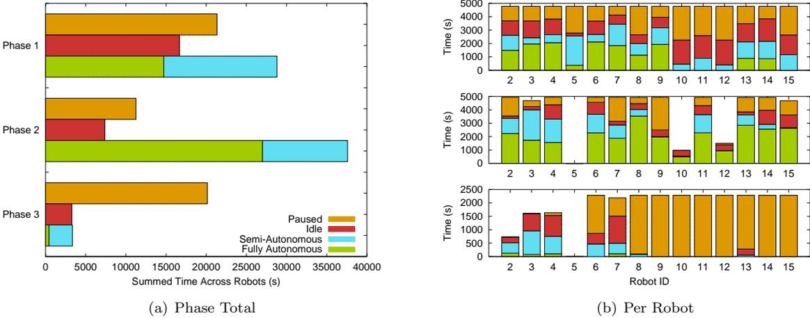
Figure 27: Time spent in each robot state during MAGIC. In (a) the combined amount of time robots spent in each mode of control is shown for each phase while (b) shows exact times for each individual robot. Shortened bars indicate robots being disabled or, in the case of robot 5, being removed from the competition due to mechanical difficulties.
