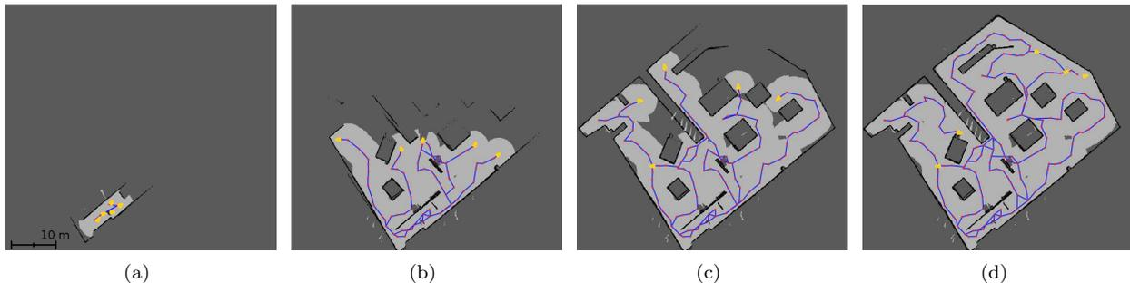
Figure 12: Robots building a trajectory graph. As the robots (yellow triangles) explore the environment (time increases from (a) to (d)), the trajectory graph (red nodes and blue traversable edges) grows into a coarse highway system. The autonomous planners use the trajectory graph to efficiently route robots long distances through explored terrain. This example was generated in a simulated  $50 \times 40$  m region.
