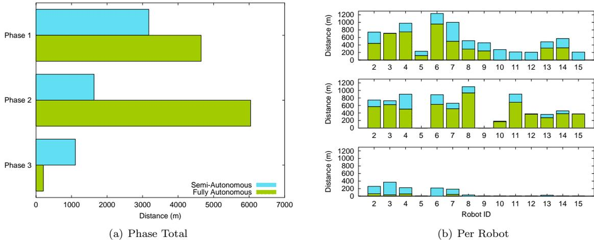
Figure 28: Distance traveled in each autonomous mode during MAGIC. (a) shows the combined distance traveled by all robots in each phase while (b) shows the distances for individual robots. Tele-operation was omitted from this figure as it was not employed during MAGIC.
