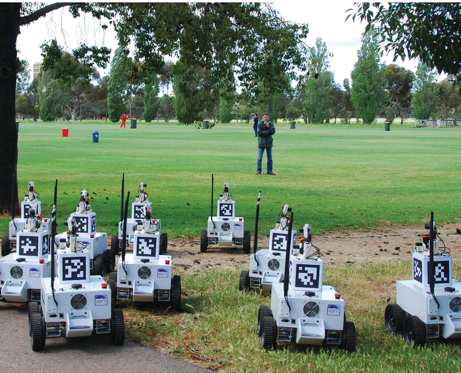
Figure 1. Team Michigan robots. Michigan deployed 14 custom-made robots that cooperatively mapped a 500m × 500m area; each included a color camera and laser range finder capable of producing 3D point clouds.
