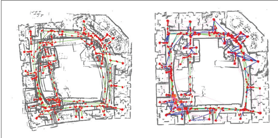
Fig. 8. Intel without front-end loop validation. Our system can identify correct loop closures and compute a posterior map from within a single integrated Bayesian framework (right); the typical front-end loop validation has been replaced with a k + 1 mixture component containing the k best laser scan matches (based purely on overlap) plus a null hypothesis. In this experiment, we used k = 5 . For reference, the open-loop trajectory of the robot is given on the left.
