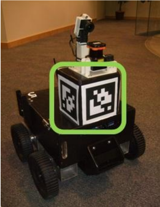
Figure 7: Robot tags. Visual fiducial markers are placed on each robot so that one robot can identify another uniquely. The ground station can build a global map from individual robot maps, when robots can place themselves relative to each other.
