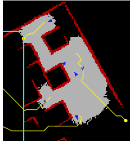
Figure 2: Exploration planning. The robots are spread across the map to avoid duplicating effort.
