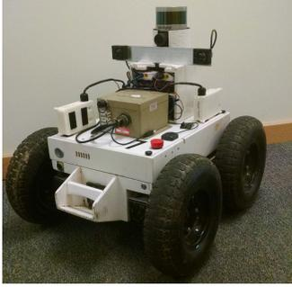
Fig. 5. April MAGIC2 robot platform used for experimental tests. The 30 cm baseline stereo camera pair is located beneath the standard monocular camera and LIDAR sensor.
