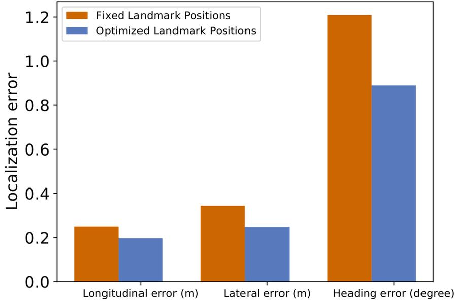
Figure 4.11: Effect of modeling uncertainty in labeled landmark positions on localization performance. Including the landmark positions reduces the longitudinal, lateral, and heading errors.
