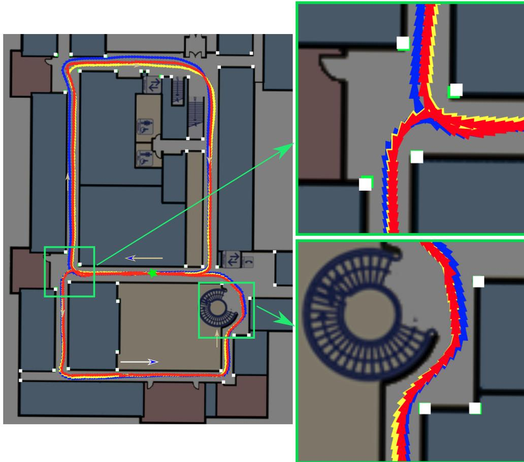
Figure 4.1: Comparison of dead-reckoning (blue), laser scan match-based localization [28] (yellow), and our FLAG method (red) over a 180 m looped path in an indoor environment. Unlike the scan matching method, FLAG uses only a floor plan with labeled corners (white squares) as a prior map, then matches vertical edge features (e.g. wall intersections) observed from the robot’s point-of-view to those landmarks. FLAG runs online for reasonable indoor speeds: here, the robot moved at about 2 m/s.
