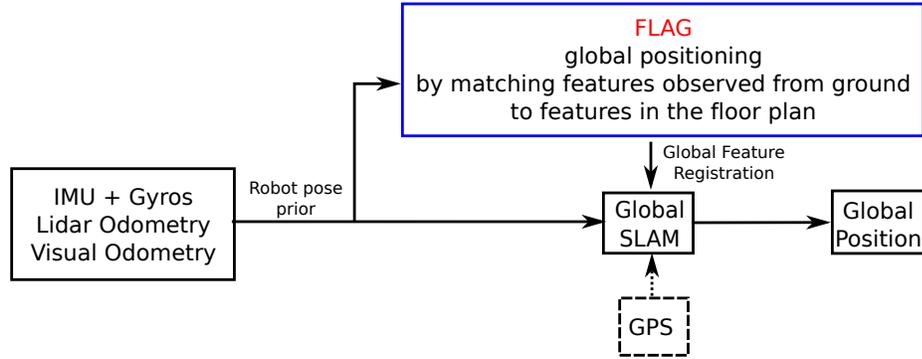
Figure 4.3: Robot localization system architecture showing the role of FLAG as a replacement for GPS.
