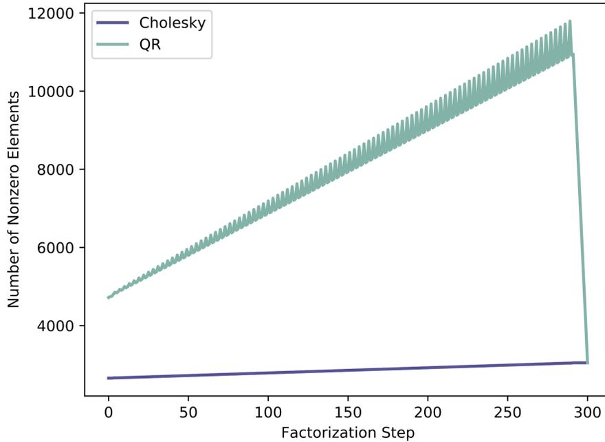
Figure 3.3: The number of nonzero elements at each step of the matrix factorization for the graph shown in Fig.3.2. QR factorization induces more nonzero elements than Cholesky during the factorization process, leading to slower computations.
