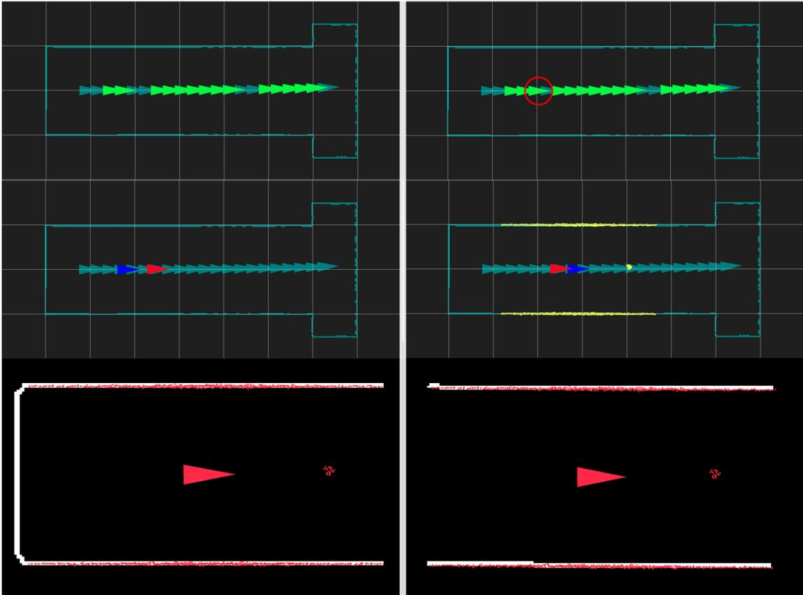
Figure 5.8: *Top left:* 14-node map selected by SSM. *Top right:* 15-node map selected by SSM. New added node is circled. *Middle:* Localization results. The red triangle is the ground truth and the blue triangle is the localized position. In the 14-node map, the robot is stuck at the beginning so it never gets chance to match scans to the rest of nodes, while adding one node in 15-node map helps the robot get out the trap.
