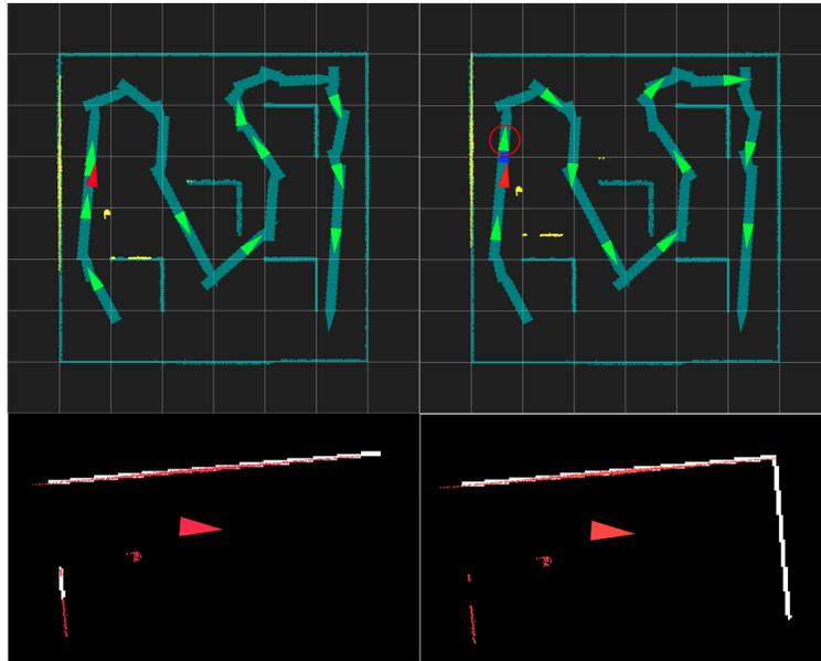
Figure 5.11: An example of Equidistant method's failure. Red triangle is the ground truth position and blue triangle is the localized position. *Left:* Robot is precisely localized in the 11-node map selected by MOSS. Map scans are shown in white and live scans are shown in red. *Right:* Robot is localized in the wrong place because of the aliasing in local view between map scans and live scans. It is pulled closed to the circled map node.
