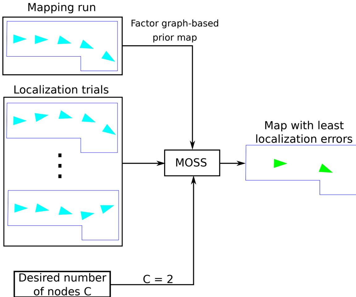
Figure 5.1: Illustration of MOSS pipeline. MOSS (Alg. 5.1) optimizes a prior map for size and saliency based on the results of localization trials, seeking to eliminate portions of the map prone to feature aliasing.
