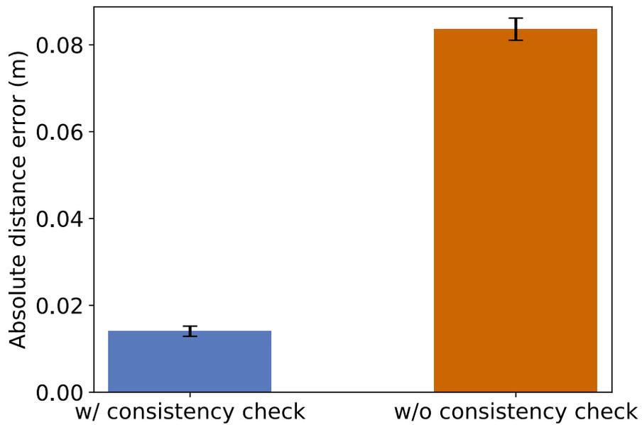
Figure 4.8: Localization error in the presence of dynamic obstacles (see Fig.4.7). Error bars represent three standard error of the mean across the 5000 trials. Using the pairwise consistency check resulted in lower error.
