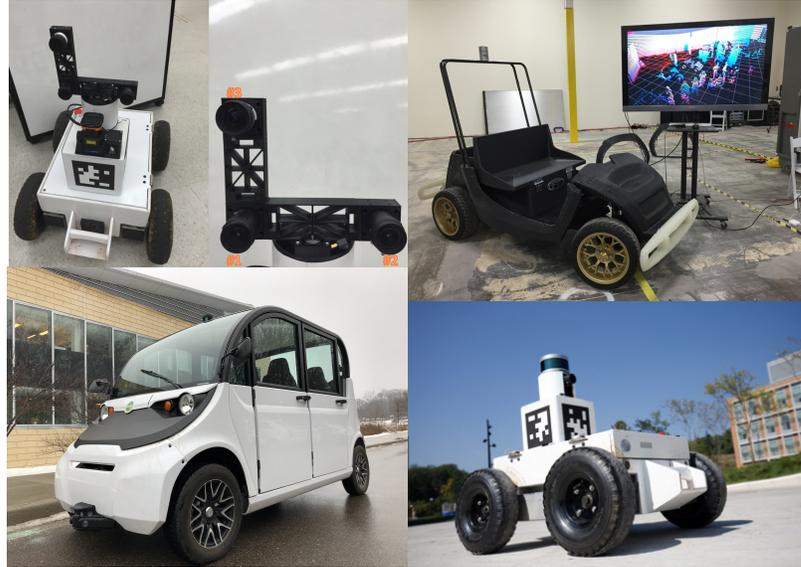
Figure 1.2: Robot applications. mapping and localization is essential for autonomous mobile robots equipped with all kinds of sensors (Lidar, cameras, radars, etc).
