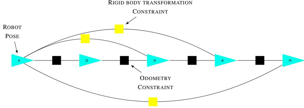
Figure 2.2: A pose graph. Cyan triangles are poses. Squares represent rigid body transformation constraint between two poses. The information matrix of this pose graph is shown in (2.24).
