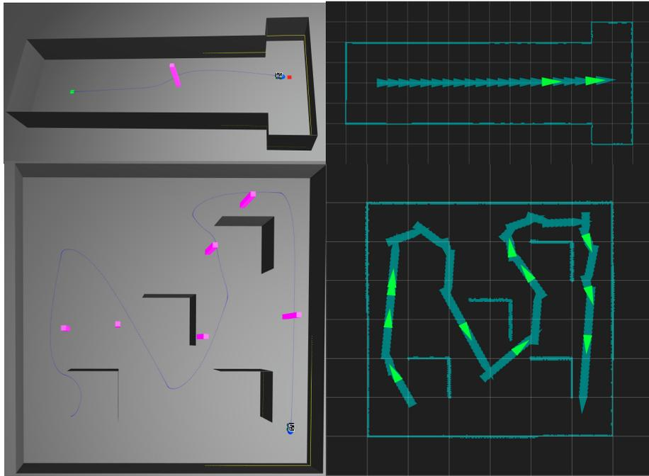
Figure 5.5: *Left*: Example localization trials in two simulated scenarios (CORRIDOR and SQUARE). *Right*: Maps produced by MOSS for both scenarios. Highlighted green triangles indicate nodes selected by MOSS from the full map to include in the map optimized for future localization performance.
