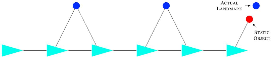
Figure 4.9: Illustration of a simulated scenario testing the max-mixture error model. The rightmost landmark is obstructed by a static object, which the robot observes instead of the landmark. For each trial, we randomly sample the location of the static obstacle within a particular radius of the landmark. We plot the localization error of the last pose in Fig.4.10.
