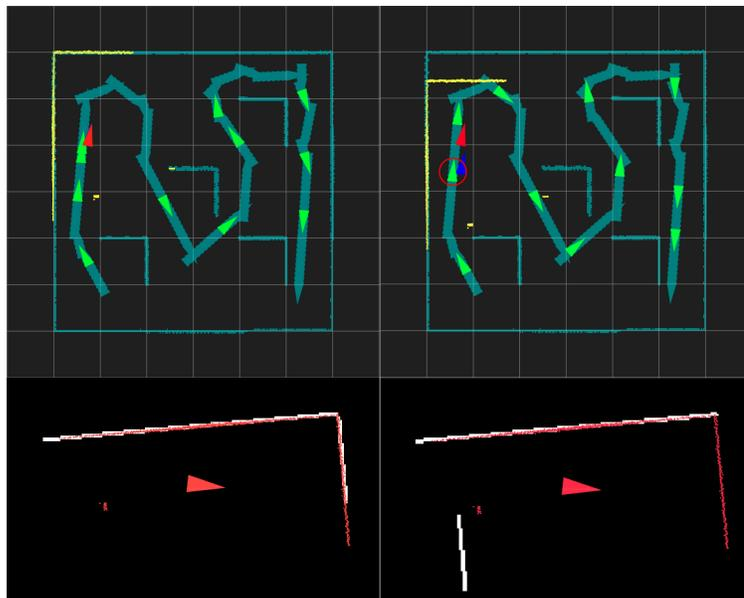
Figure 5.12: An example of SSM method's failure. Red triangle is the ground truth position and blue triangle is the localized position. *Left:* Robot is precisely localized in the 11-node map selected by MOSS. Map scans are shown in white and live scans are shown in red. *Right:* Robot is localized in the wrong place because of the aliasing in local view between map scans and live scans. It is trapped near the circled map node.
