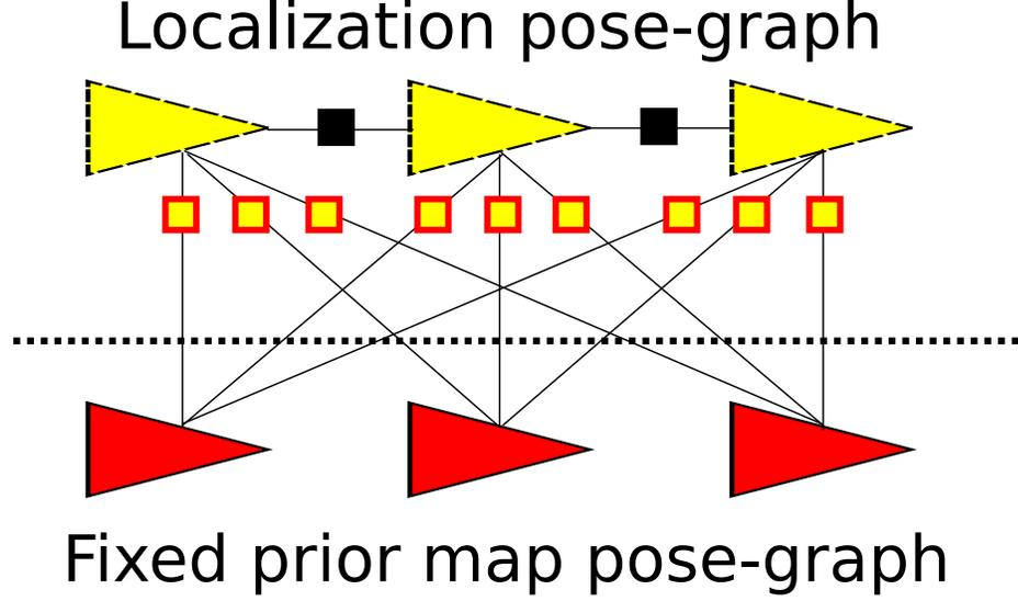
Figure 5.4: A simple example of a factor graph for localization. Yellow triangles are localization nodes and red triangles are map nodes. In addition to standard factors based on inertial measurements (black squares), scan matching factors (yellow squares) are added describing transformations back to a known map (in red). During optimization, the portion of the graph corresponding to the known map is held fixed.
