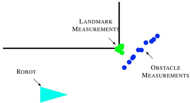
Figure 4.7: Illustration of simulated test of the pairwise consistency check algorithm. Green dots show the 10 measurements of the landmark, which are sampled from its true location with variance 10 cm. The blue dots show observations of a dynamic object moving along a straight line, from which measurements are sampled with variance 1 cm. The results are shown in Fig.4.8.
