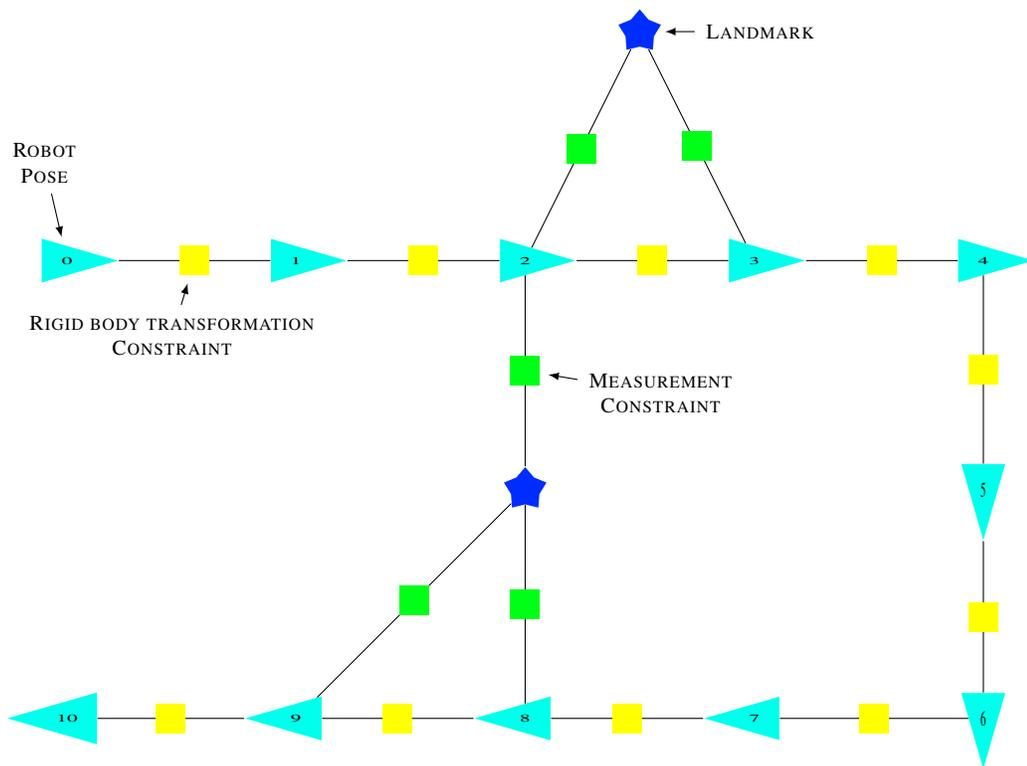
Figure 2.1: Sample pose/feature graph. The robot trajectory is discretized into a series of poses (cyan triangles) from which the robot observes landmarks (blue stars). Both poses and landmarks are nodes in the graph. Graph edges represent constraints between the two nodes, and squares represent the probability factors.
