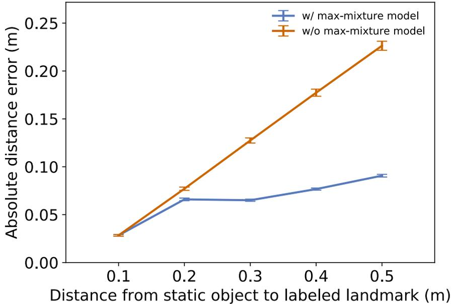
Figure 4.10: Localization error in the presence of a static obstacle. Error bars represent three standard error of the mean across the 5000 trials. As the static object gets further from the true landmark localization, the effect of using the max-mixture model becomes more pronounced.
