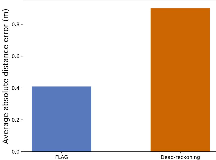
Figure 4.6: Average absolute distance errors of FLAG and dead-reckoning over a 180 m looped path in an indoor environment for 4 different runs (Fig.4.1 shows one of four runs). We use a state-of-the-art laser scan match-based method (with a Lidar prior map) as an approximate ground-truth.
