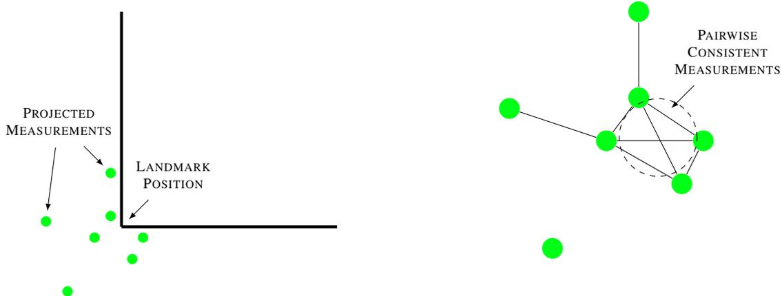
Figure 4.5: Illustration of the pairwise consistency check. The green circles (*left*) are the projected positions of landmarks based on distance and bearing measurements. These measurements form an undirected graph (*right*). Edges exist between nodes if the projected landmark positions from the two measurements are within a threshold distance. A clique in the graph represents a set of internally consistent measurements. We reject measurements that are not part of a sufficiently large clique.
