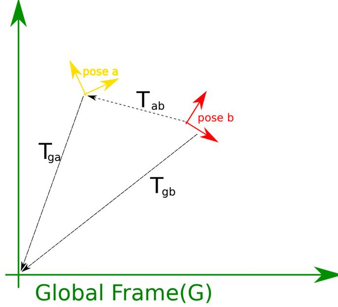
Figure 2.3: Coordinate transformations. Each robot pose represents a local coordinate system which can be related to the global coordinate by a rigid-body transform. Two local coordinate systems can also be related, e.g.,  $T_{gb} = T_{ga}T_{ab}$ . Point  $P$ , expressed with respect to coordinate frame  $B$ , can be projected to coordinate frame  $A$  by  $T_{ab}P$  and to the global coordinate frame by either  $T_{gb}P$  or  $T_{ga}T_{ab}P$ .
