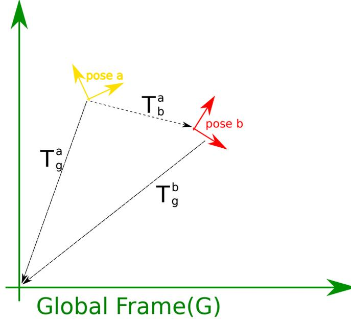
Figure 5.3: Coordinate transformations. Each robot pose represents a local coordinate system that can be related to the global coordinate by a rigid-body transform. Two local coordinate systems can also be related, e.g.,  $T_g^a = T_b^a T_g^b$ .
