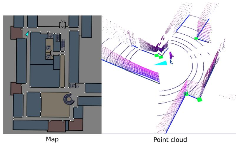
Figure 4.2: FLAG performs global localization in a previously unvisited environment. It uses a floor plan (*left*) as a prior map with labeled corners (white squares) as landmarks. The robot extracts vertical features from a 3D point cloud (*right*) and matches those features (green squares) to the landmarks in the prior map. It adds the robot’s discrete poses and the landmark positions to a factor graph to be optimized.
