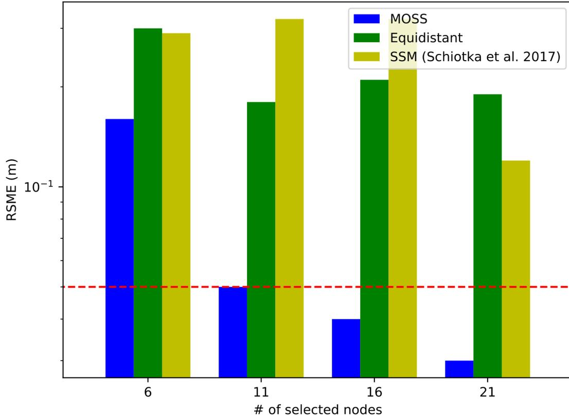
Figure 5.9: Localization test results in SQUARE. The red dashed line is the localization performance using the original map (i.e.  $C = 204$ ). MOSS achieves the best localization results across each tested map size. MOSS achieves localization performance at least as good as that of the original full map with as few as  $C = 11$  nodes, a reduction of approximately 95 percent in map size.
