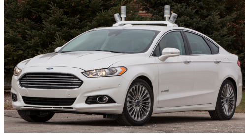
Fig. 2. Our autonomous car platform, a Ford Fusion equipped with four LIDAR units, survey-grade INS, and a single forward-looking camera. All control and perception is performed onboard.
