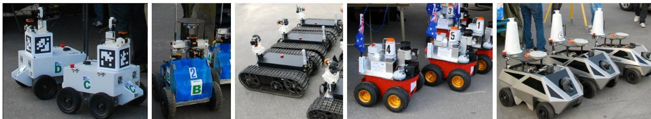
Fig. 2. Finalist robots. Each team used a unique robot platform (left-to-right, in ranked order): Team Michigan used 14 custom-built robots; University of Pennsylvania fielded 7 custom robots; RASR based its 7 robots on the Talon commercial platform; Magician adapted a commercial base for its 5 robots; Cappadocia built 6 tailored vehicles.
