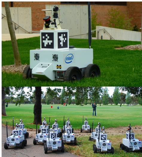
Fig. 1. Team Michigan Robots. We deployed fourteen custom-made robots that cooperatively mapped a  $500 \times 500\text{m}$  area. Each robot had a color camera and a laser range finder capable of producing 3D point clouds.
