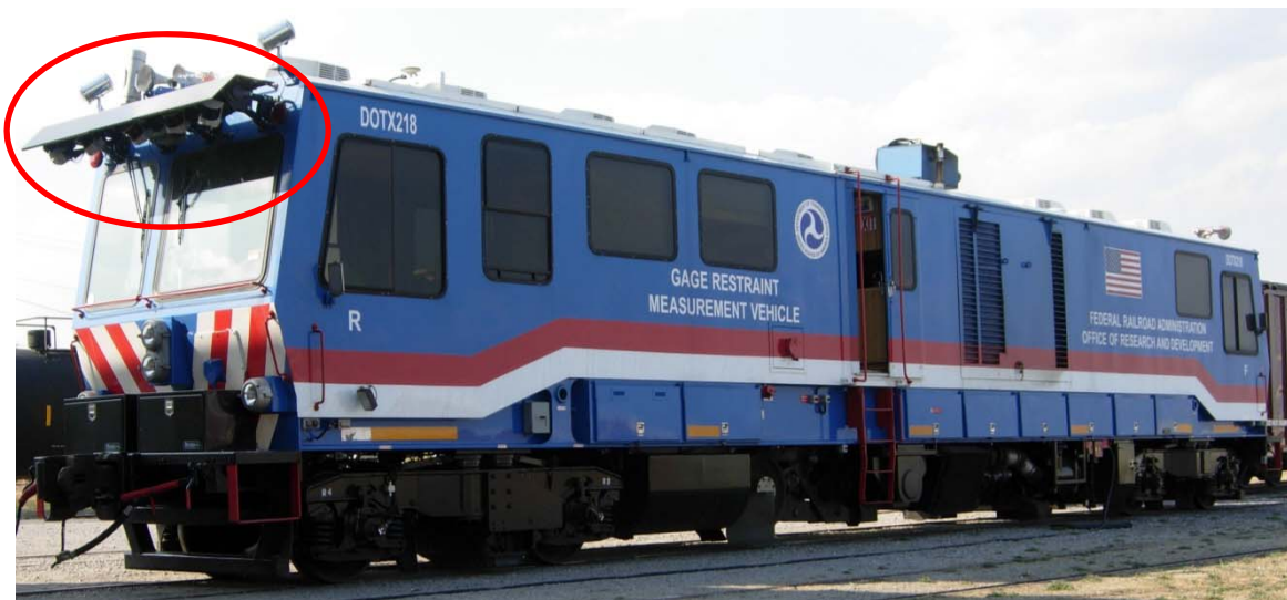
Figure 1. FRA's LiDAR-Based Surveying System on DOTX 218
